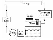
**Fig. 3.** The principle scheme a filtration system [2]
