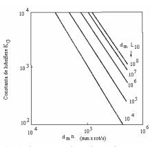
Fig. 1. Constant value when using grease lubrication [1]
